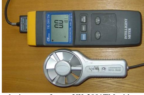
Figure 10. Air flow velocity meter LutronYK-2001TM with anemometer AM-04
