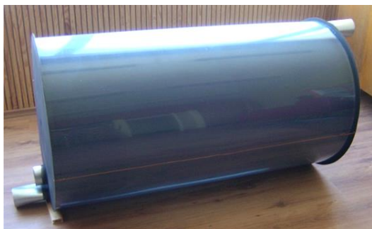
Figure 8. Cylindrical solar collector for air heating.
