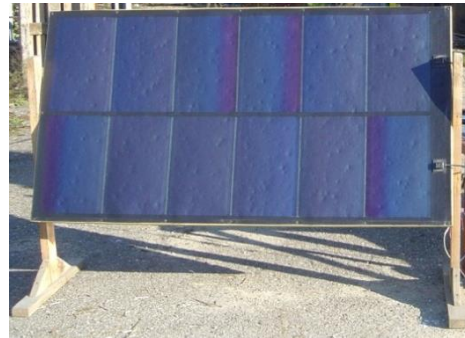
Figure 2. An amorphous silicon flexible PV module 19V; 97W.
