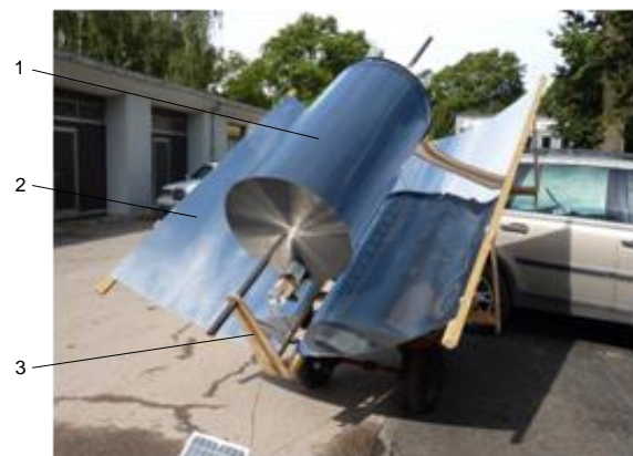
Figure 9. Cylindrical solar collector device: 1 – solar collector; 2 – solar radiation concentrator; 3 – frame.
