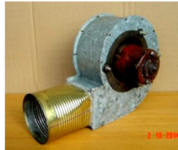
Figure 4. Centrifugal ventilator with direct current electric motor: 12 V; 4.5 A.
