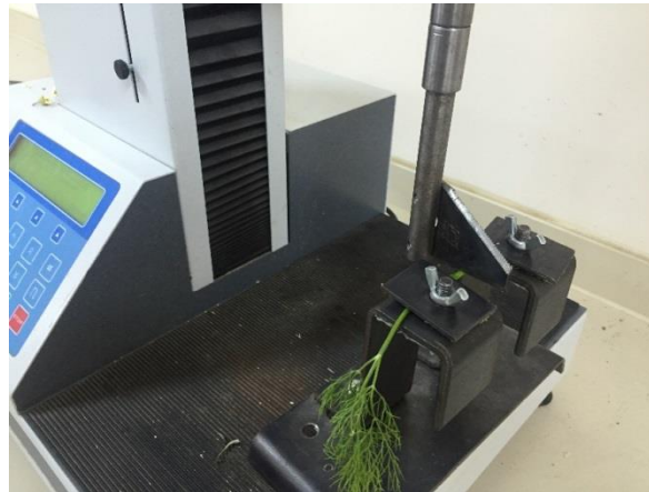
Figure 2. Computer-aided systems for measuring the cutting of dill ( Anethum graveolens L.) plant
