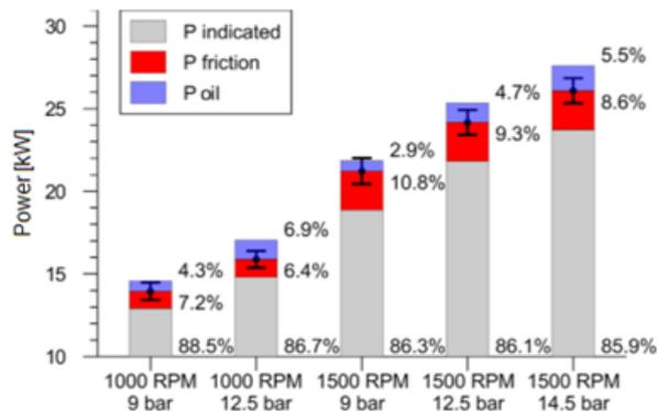
**Figure 4.** Compressor energy balance at different operating points (percentage refers to the mechanical power) [2]
