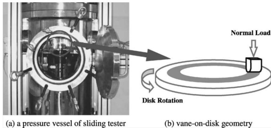
**Figure 9.** High pressure wear tester [7]
