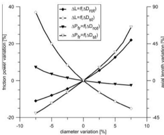
**Figure 7.** Influence of the aspect ratio on the compressor geometry and friction power dissipated [6]
