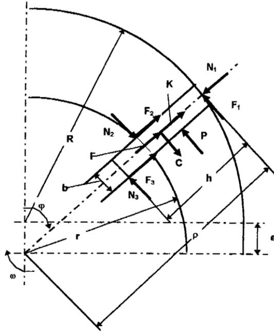
**Figure 2.** The forces that are acting on the single vane [5]
