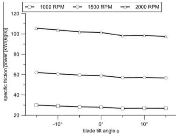
**Figure 8.** Variation of the friction power per unit air delivered with revolution speed and blade tilt [6]
