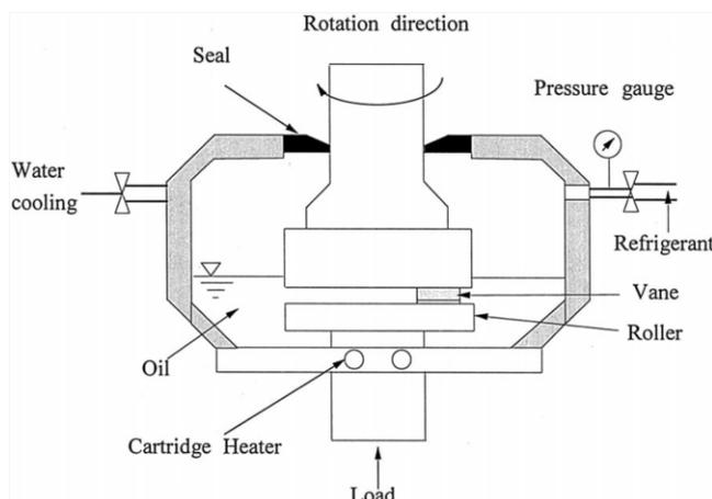
**Figure 12.** Schematic diagram of Falex wear test machine with high pressure chamber [8]
