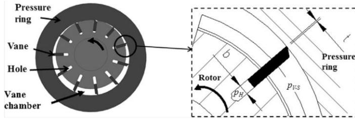
**Figure 14.** Sketch of the pressure ring (stator), rotor, vanes and holes [9]
