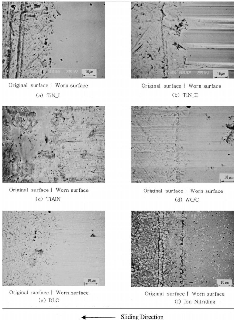
**Figure 13.** SEM pictures of the wear on the vane tip for various coatings. (a) TiN(I)-; (b) Tin(II)-; (c) TiAlN; (d) WC/C; (e) DLC; (f) ion nitriding in R407C and POE oil mixture tested in normal load of 440 N, speed of 350 rpm, 708C, and tested duration of 10 h. [8]
