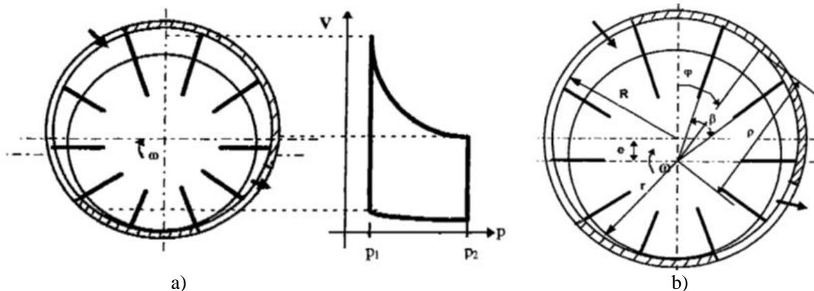
**Figure 1.** The construction scheme and the compression process for vane type rotary compressor a) the main construction dimensions b) [5].
