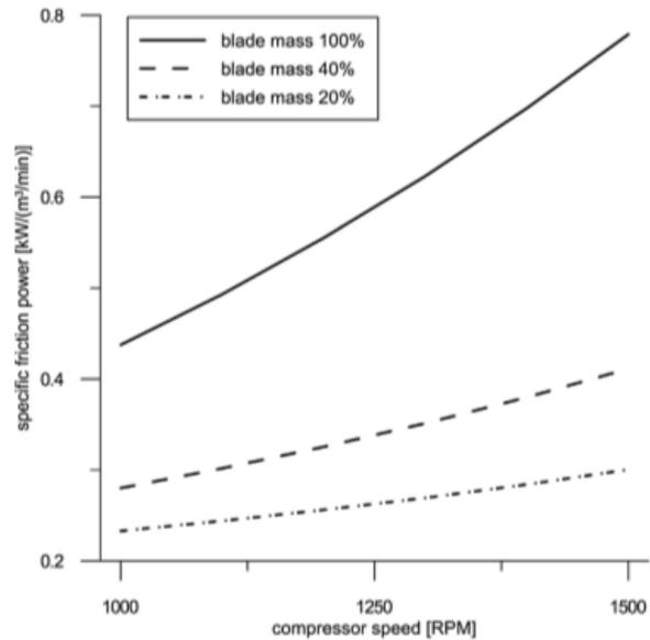
**Figure 5.** Effects of blade mass and revolution speed on the specific friction losses compressor operating at 12.5 bar [2]
