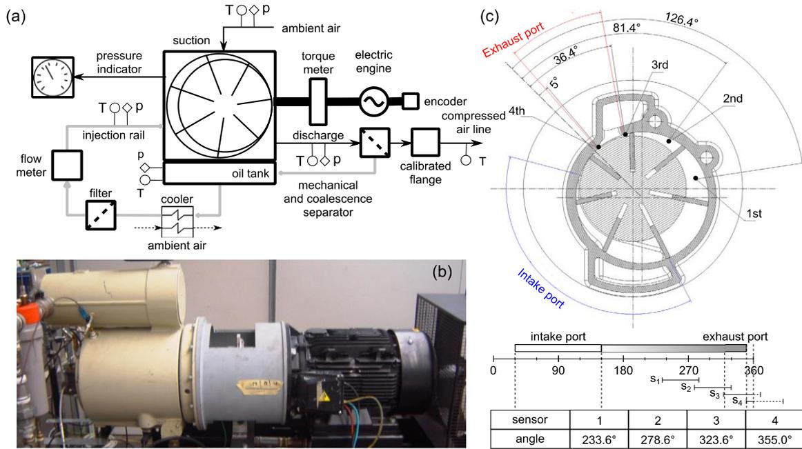
**Figure 6.** Experimental setup – transducers layout (a), test bench (b), piezoelectric sensors positioning (c). [6]
