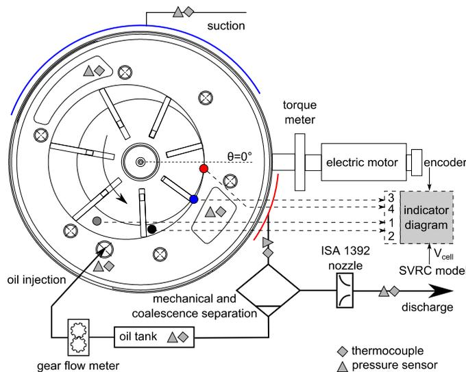
**Figure 3.** Experimental setup. Compressor Mattei ERC 22L [2].
