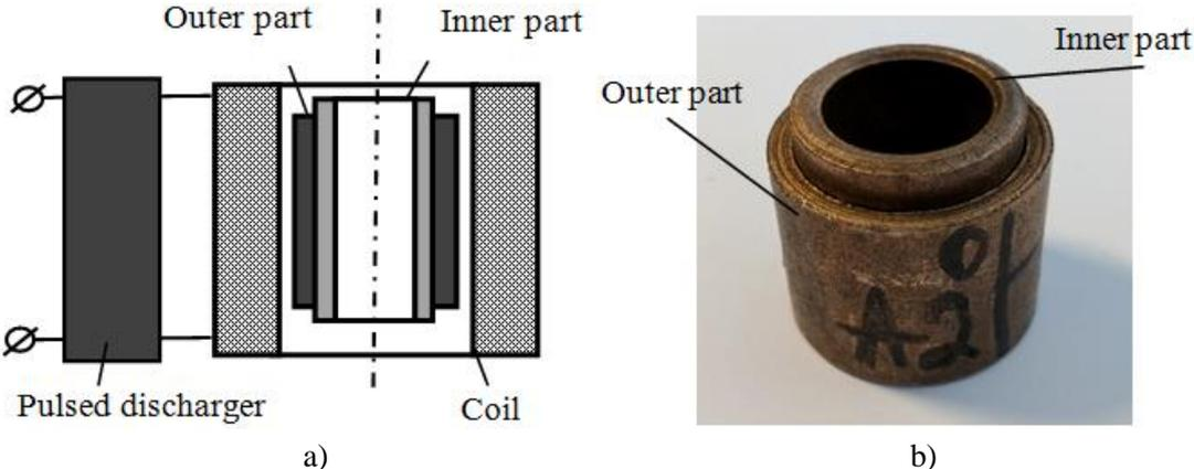
**Fig. 1.** Principle schematic of PMD crimping a) and bushing-bushing joint view obtained by PMD b).
