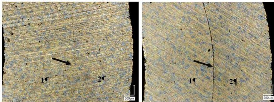
**Fig. 3.** Samples of joints fragments showing tight (left) and weak (right) PMD crimping: 1 – inner bushing; 2 – outer bushing; arrows show boundary between inner and outer parts.
