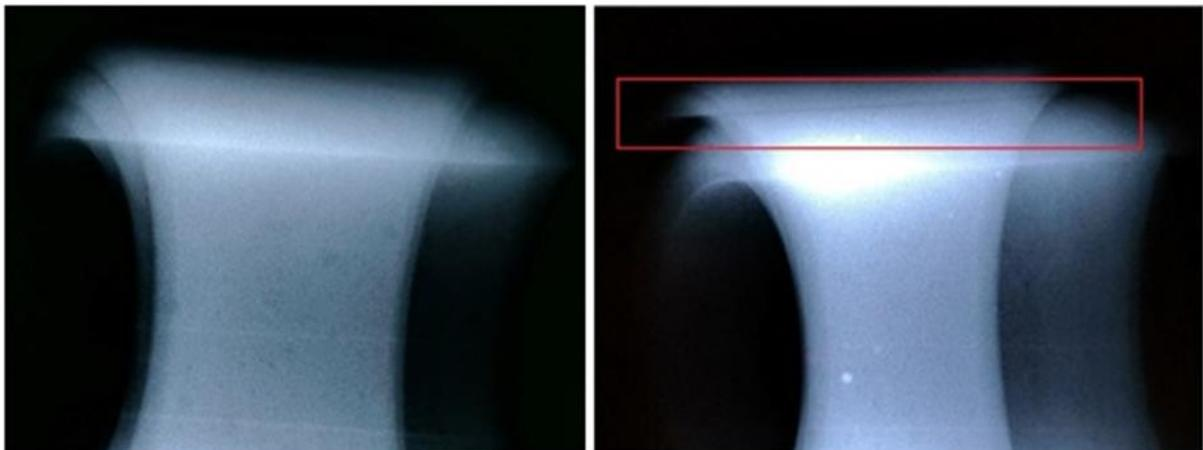
**Figure 6.** The same as in Figure 5, axial view. Images obtained at an angle approximately  $30^{\circ}$ . Rectangle shows the gap of improper crimping.
