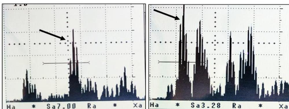
**Fig. 4.** Samples of ultrasonic echograms showing cases of tight (left) and weak (right) PMD crimping. Arrows show reflections corresponding to 7.00 and 3.28 mm thicknesses in these cases, i.e. from double and single walls.
