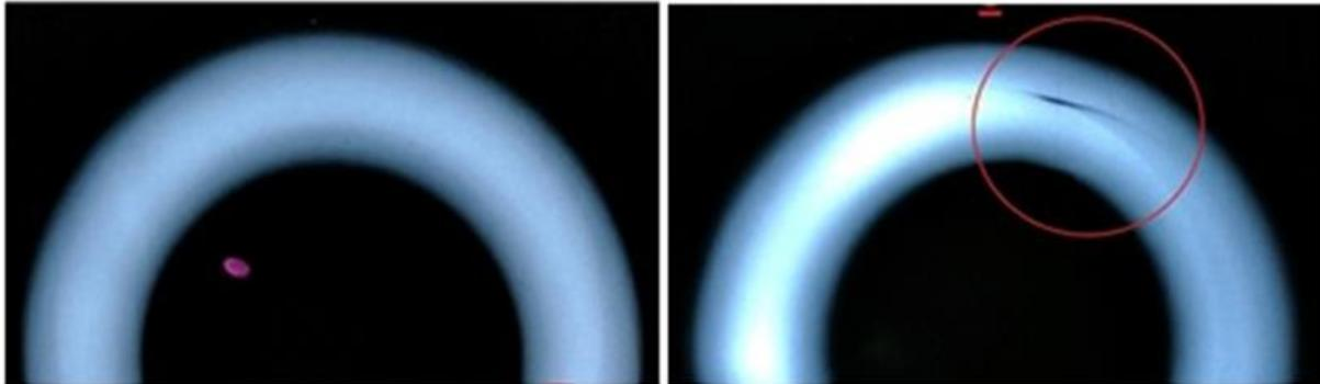
**Fig. 5.** Samples of X-ray films showing cases of tight (left) and weak (right) PMD crimping for bushing-bushing joints. Circle shows the area of improper connection. Images obtained from the end face of bushing.
