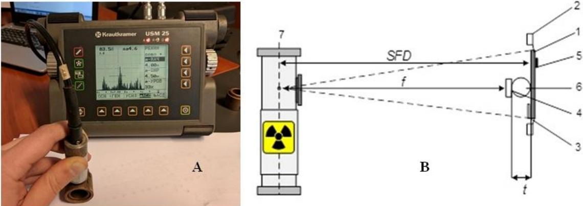
**Fig. 2.** Ultrasonic(A) and radiographic (B) testing of bushing-bushing joint: 1 – lead shield; 2 - film; 3 and 4 – marks of object and reference point; 5 – indicator of back radiation; 6 – object; 7–x-ray source; f – distance between source and object; SFD – source-film distance; t – object thickness.
