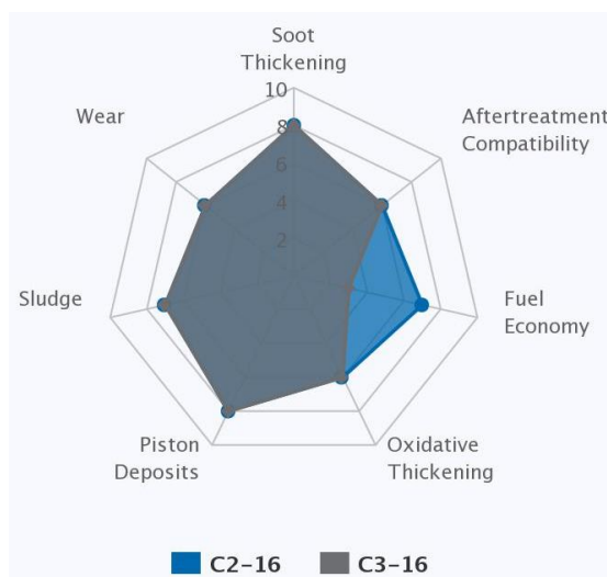
Figure 1. Performance of investigated engine oils according to Lubrizol relative performance comparison tool (Lubrizol, 2016)
