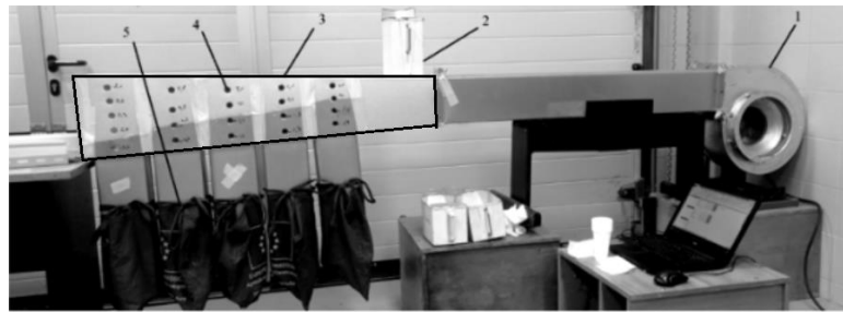
Fig. 1 Research stand: 1 - fan; 2 – grain seed box; 3 - grain sorting chamber; 4 - air flow velocity measuring hole; 5 – collection bag
