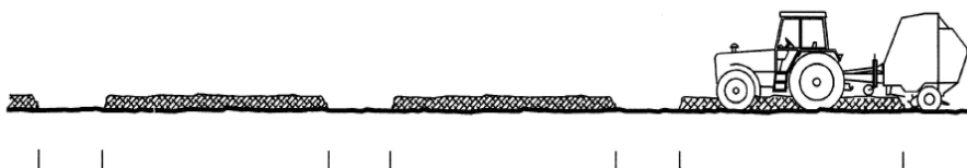
Fig. 2. Calibration line – 10 m row + 5 m space
