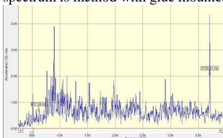
Fig. 4. Acoustic signal spectrum of the turbocharger in frequency range from 0 kHz to 4 kHz
