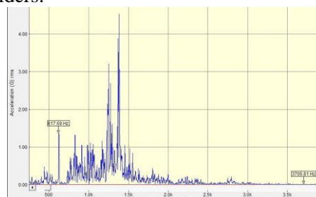
Fig. 5. Vibration signal spectrum of the turbocharger in frequency range from 0 kHz to 4 kHz – magnetic sensor holder
