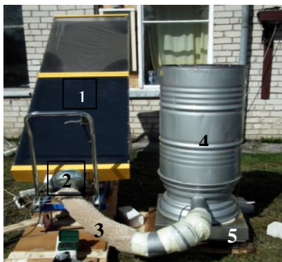
Fig.1. Drying equipment with mobile air heating solar collector: 1 - modular solar collector with variable angle setting; 2 – fan; 3 – air inlet; 4 – drying equipment; 5 – scales.
