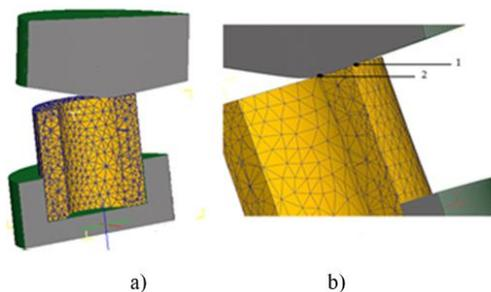
**Fig. 10.** The finite element method of RS flanging modeling for the outer clamp on the tube workpiece: a) calculation model; b) the location of the calculation points 1 and 2 [11].
