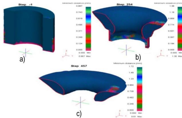
**Fig. 9.** Changing the maximum distance between the plane of the mandrel and the surface during the stamping process: a - the appearance of the workpiece before the RS; b - the workpiece on the 254 step of the RS process modeling; c - workpiece at the final stage of simulation.
