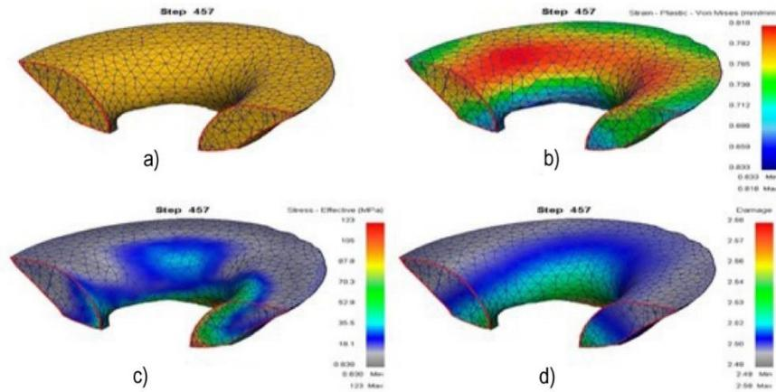
**Fig.18** Analysis of VAT modeling results: form change a); distribution in the midiary section of the pipe workpiece at the final stage of the RS accumulated deformation b); intensity of stress in); accumulation of damage d).
