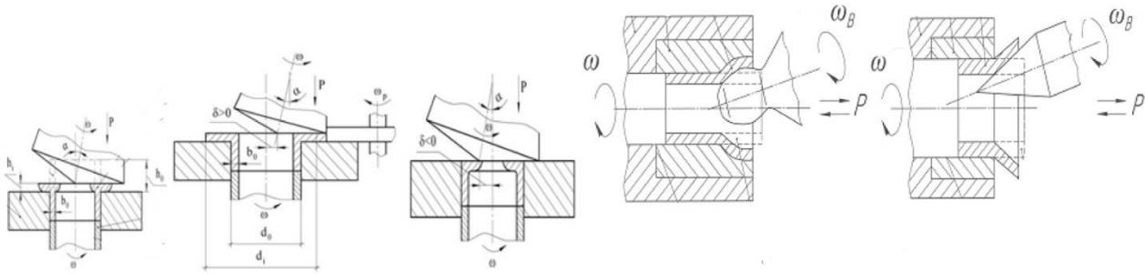
**Fig. 2.** Influence of the direction of displacement of the peak of the roll of the axis of the workpiece on the shape change of the workpiece during the loading of the clamps by the method of RS
