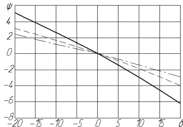
**Fig. 3.** Dependence of the angle  $\psi$  from the direction and the displacement value  $\delta$  at different angles of the cone:  $\alpha = 2^\circ$  (solid line),  $\alpha = 10^\circ$  (dashed line),  $\alpha = 20^\circ$  (dashed-dotted line).
