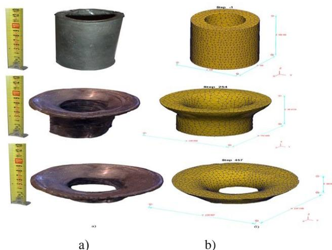
**Fig.14** RS of a lead workpiece №5: a) experimental research; b) modeling in DEFORM 3D[7].
